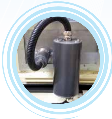
After DRYING and SCREENING Measurement of SURFACE and CORE Layers Moisture range: 0.5% to 5%
