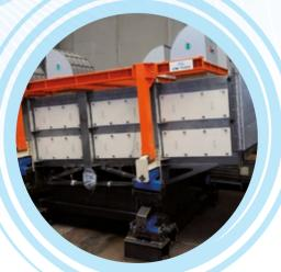
A group of REMBE "Q-Box units" is located on the upper section of the screening machine, instead of the traditional bursting panels. Their function is: to allow gradual venting in case of an explosion and to mitigate the pressure wave arising from the explosion itself. In this way, the flames and pressure wave will be reduced to non-critical-effects inside buildings, and the safety distances to be kept around the machines will decrease as well.
